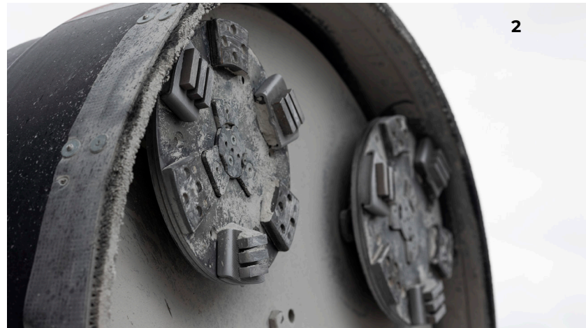
1 Digital display | 2 Grinding head with mounting plate and diamond tools
